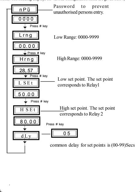
**Special Note:** The decimal point can be changed by pressing shift button for five times the decimal point starts to flash. Now press increment button to change the place of decimal point as need and press enter button to save.
