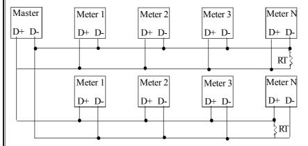
In this method termination resistor RT (60 -100 W) of value equal to characteristic Impedance of the cable used may be required to avoid reflection loses.
