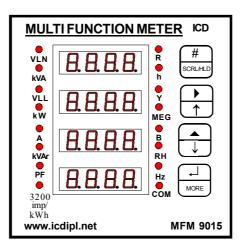
The LED Display is a 4 row 0.56" quard digit 7 segment red display. It is used to display voltage, current, kVA, kW, KVAr, PF, Freq., kWh, kVAh, kVArh, Run Hour, THD(if applicable) & program mode settings.
